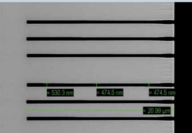
Sub-micron trenches with high aspect ratio etched into single crystalline Si.
