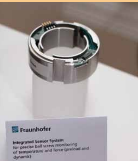
Integrated sensor system for precise ball screw monitoring of temperature and force.
