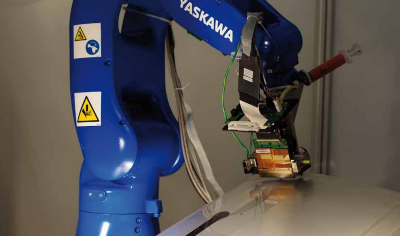
Fabrication of functional layers by means of a 6-axis-robot-assisted inkjet printing technology for the manufacturing of cable harnesses on car parts.
