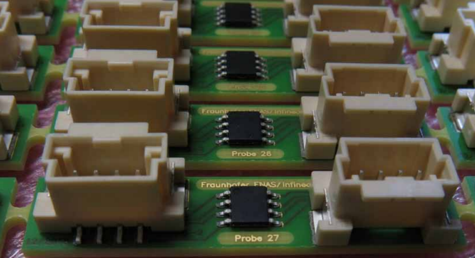
DIL 8 (dual in line) package with implemented stress measure chip for in situ analysis of process and lifetime conditions.
