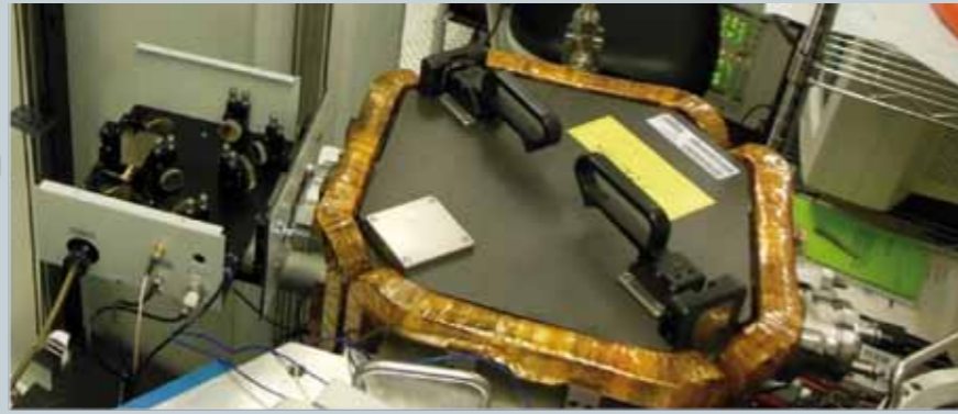
Schematic and photographic representation of a modified process chamber with connected multi-pass optics (MPO) for plasma analysis by means of QCLAS.
